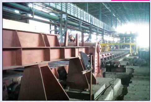
BRG Plate Mill in operation for plate thickness 8mm & above, Widths 1250 - 2050mm
