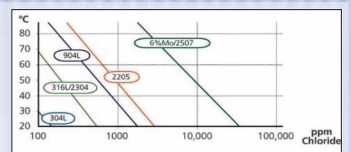
Figure 1 Maximum temperatures & chloride contents to which stainless steels are resistant in water with residual chlorine of about 1ppm. Reproduced from data sourced from Outokumpu.
