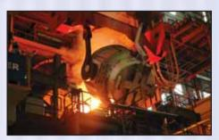
Charging Liquid Steel into AOD Converter
